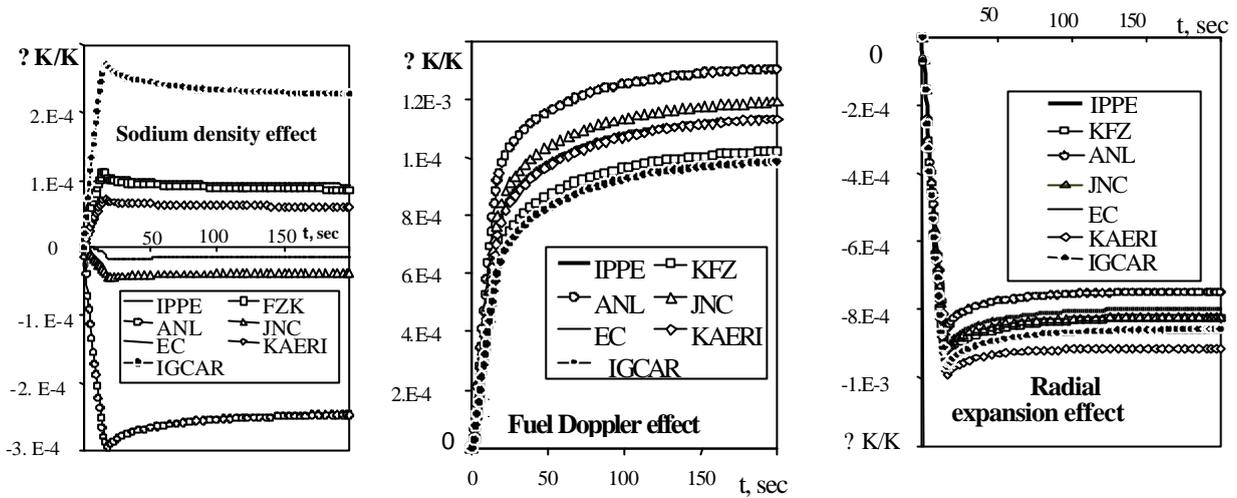
Fig. 10. Change of basic feedback reactivity components in ULOF accident
