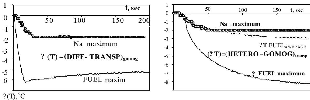
**Fig. 12.** Influence of transition from diffusion to transport approach and heterogeneous corrections to the description of ULOF accident (based on the FZK/IKET result)
