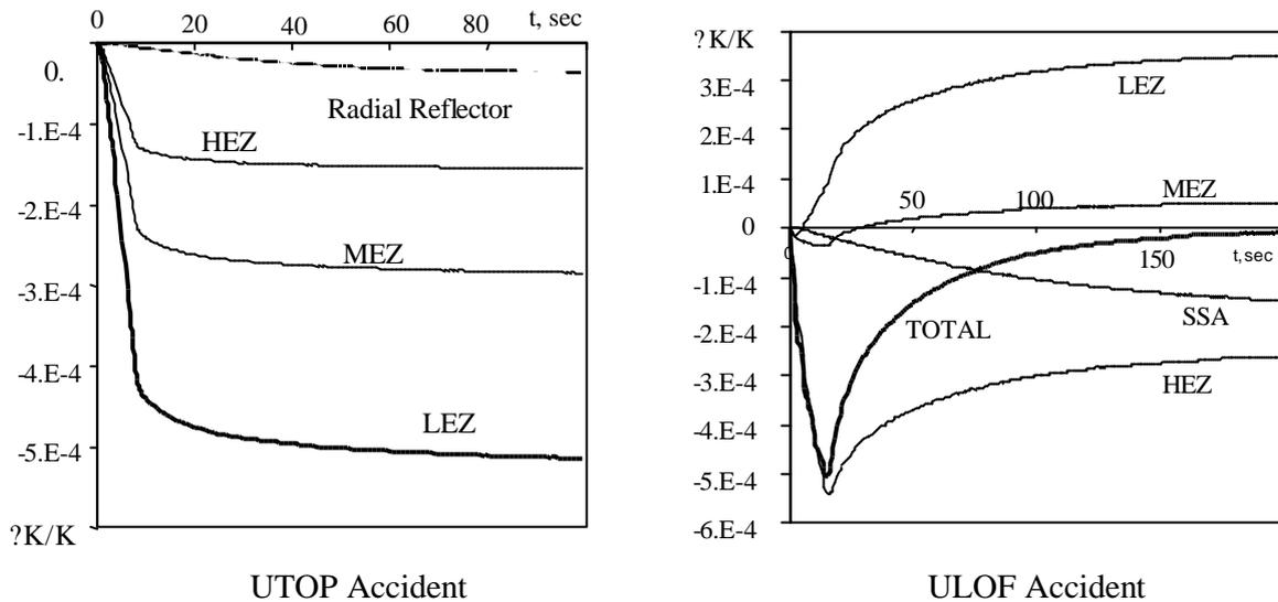
**Fig. 8.** Contributions of various fuel zones to total reactivity (diffusion approach, HEX-Z model)
