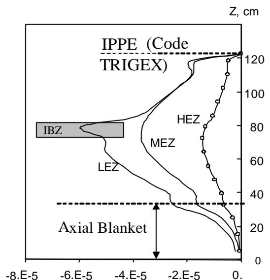
Fig. 4. Axial distribution of the fuel Doppler coefficient (for  $\beta_Z = 1$  m) (IPPE result)
