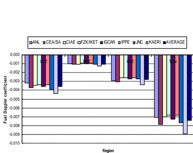
Fig. 3. Fuel Doppler coefficient
