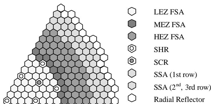
**Fig.1** Layout of BN-600 full MOX core model (60° sector, rotational symmetry)
