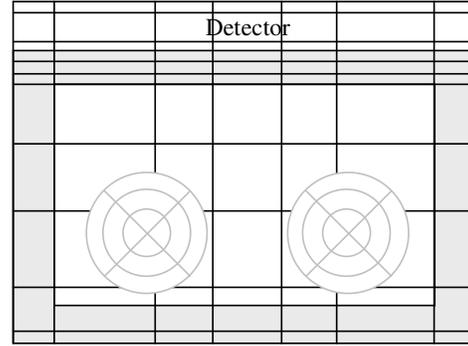
The MULTIMAP feature allows multiple importance maps to be specified in a MCBEND calculation. The MULTIMAP feature therefore allows the R $\theta$ Z mesh (light grey) in the source drums to be defined independently of the XYZ mesh over the remainder of the problem.
